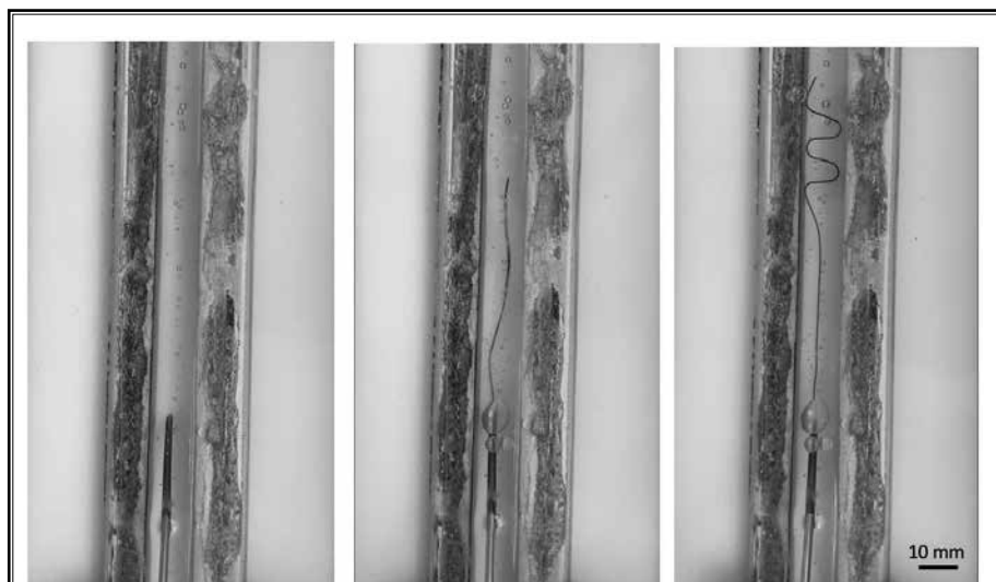
Fig. 5. Successful deployment of proposed design into a model epidural space. 1) Insertion of sheathed nitinol; 2) removal of sheath from nitinol; 3) recovery of nitinol into trained shape.
