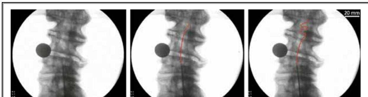
Fig. 7. X-ray fluoroscopy images of the same procedure from Fig.6 and a quarter for reference with the nitinol highlighted over in Red. 1) insertion of sheathed nitinol, 2) removal of sheath from nitinol, 3) recovery of nitinol into trained shape.
