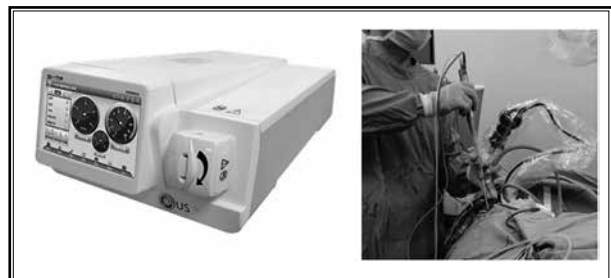
Fig. 2. The endoscopic-matched ultrasonic osteotome device includes a host machine (left) and a handpiece (right), which connects with the host and controls the disposable tips.
