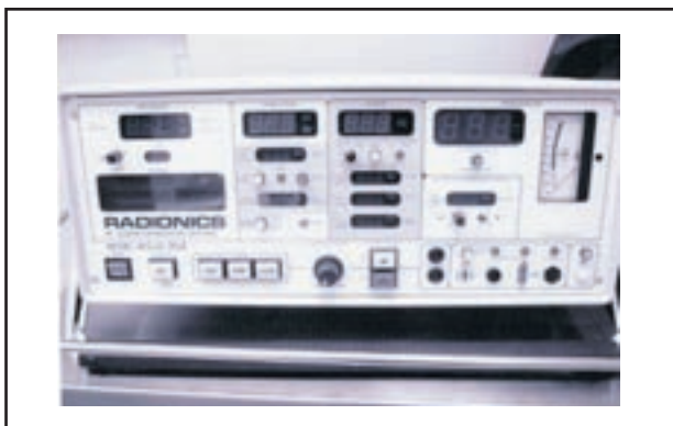
Fig. 4. Picture of the Radionics RFG-3C+ radiofrequency lesion generator which has a 50 Hz stimulator with adjustable voltage. (Radionics copyright 2001-2002 by Tyco Healthcare Group LP “Tyco”).
