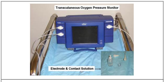
Fig. 1. The transcutaneous oxygen pressure monitor, TCM400 (Radiometer, Copenhagen, Denmark), with electrode and contact solution.
