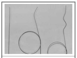
Fig. 2. Curved mandrel and "snake" mandrel, both made of Nitinol\*, to be introduced into the LisiJect RF++ catheter to direct it (curved) or to increase the mechanical lysis area, at the end of radiofrequency treatment (snake).
